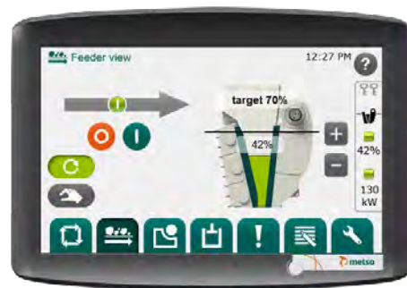
IC10C crusher automation for crushing process optimization and monitoring.
