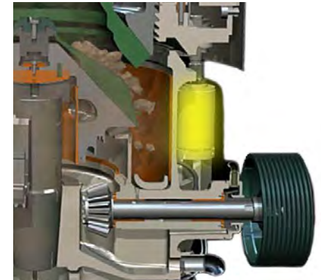
Tramp release system with large clearing stroke for quick, safe and easy cavity clearing in case the crusher stops under load for any reason
